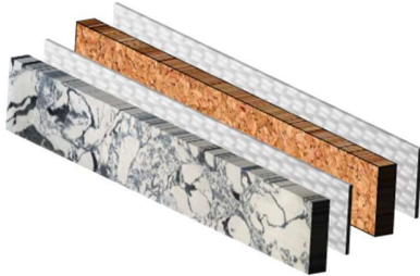
Figure 1.1 Exploded view of the material layers of the composite
