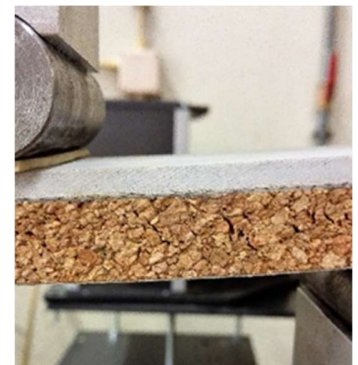
Figure 3.5 Macro-cracks on the cork layer on the fatigue tests with resting time
